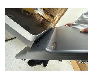
Lock the base onto the signage. During installation, you can first place it on a desk or a flat surface, then turn the signage over with the front facing upward and align the three screw holes at the bottom as shown in the picture.
