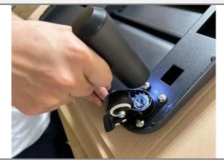
During installation, please make sure with the brake plate facing outward before installing the screws.
